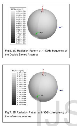
The gain of this double slotted antenna is 2 dBi. The simulated radiation patterns of the designed antenna at 1.4 GHz and 9.65 GHz resonant frequencies are shown in fig-4 and fig-5 respectively. Simulated 3D radiation pattern at 1.4 GHz and 9.65 GHz are shown in fig 6 and fig 7.
